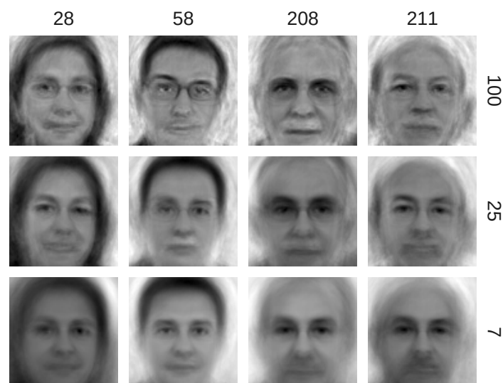
Figure 6.12: Reconstruction from a PCA that never saw the faces shown (fit on the other 344), keeping 100 / 25 / 7 components. Labels are the file numbers in index.csv .
