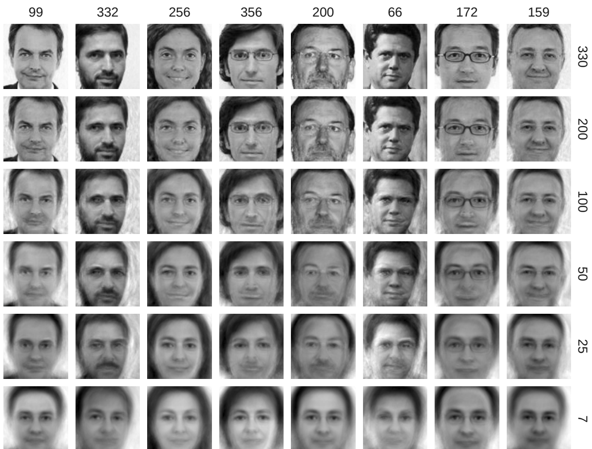
Figure 6.11: Reconstruction of eight representatives keeping comps principal components: full model (330) down to 7. Labels are the file numbers in index.csv .
