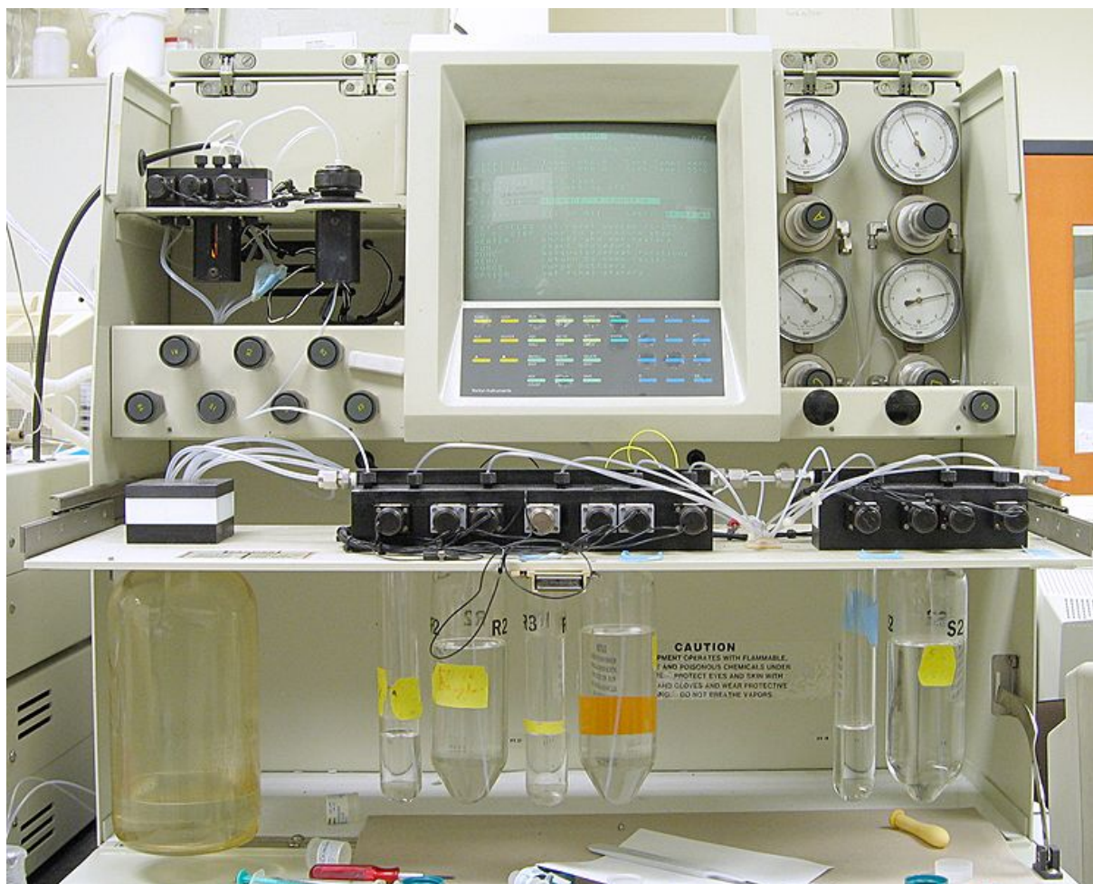
Figure 5.5: A Beckman-Coulter Porton LF3000G protein sequencer.
